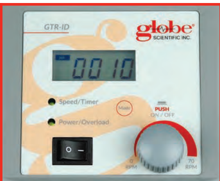
Digital display of the GTR-ID can be accurately set using the parameter adjustment knob
