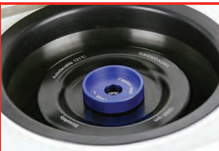
Included biosafety aerosol containment lid
